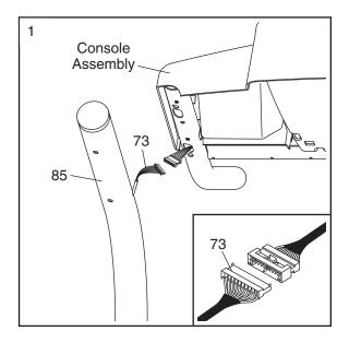
2. With the help of a second person, set the console assembly on the Uprights (85). **Make sure that no wires are pinched.** Attach the console assembly with four Console Bolts (72), Washers (96), and Star Washers (67) (only one side is shown). **Start all four Bolts before tightening them.**
